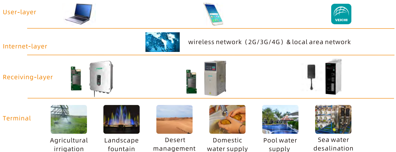
Photovoltaic pump IOT topology diagram
