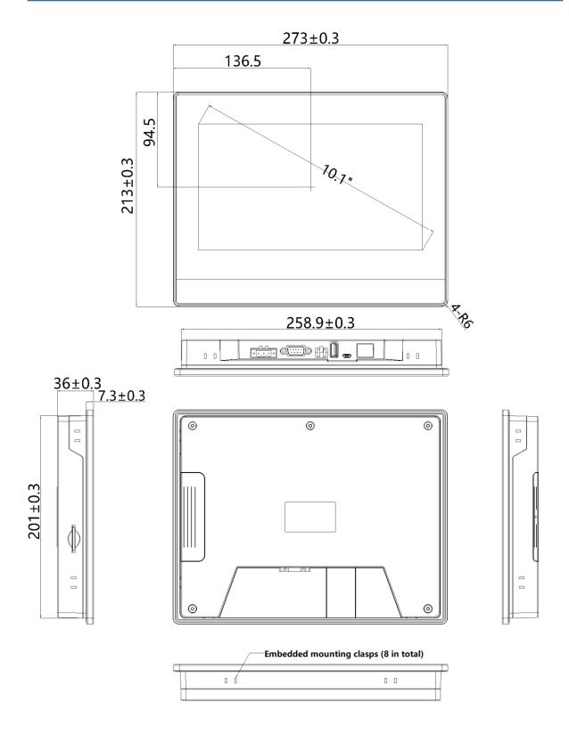
Embedded installation opening size: 260 \* 202 (+ 1.0 mm / - 0.0 mm)
