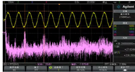
Turn off the spectrum analysis of random carrier frequency
